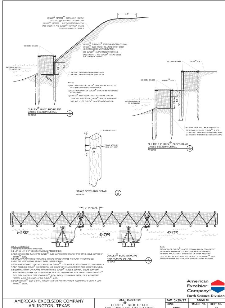
CURLEX® BLOC DETAIL FOR SHORELINE APPLICATIONS SCALE PROJECT NO. SHEET NO. NONE 23
