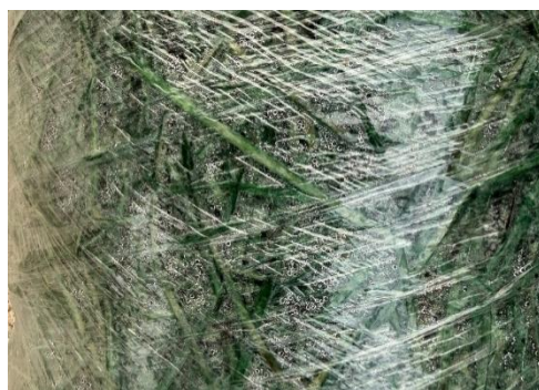
4a & 4b. Mold growth in a competitor's excelsior blanket, including visible dark mold within the fibers. American Excelsior Company minimizes this risk through strict quality controls. Curlex ECBs with QuickGRASS® use an environmentally friendly, malachite-green-free pigment applied to naturally dried Great Lakes aspen fibers. The dry fibers promote even color distribution and help prevent mold growth when properly stored.
