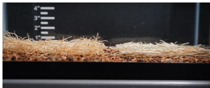
5. Curlex aspen excelsior fibers (left) expand more when wetted than competitor's excelsior fibers (right).
