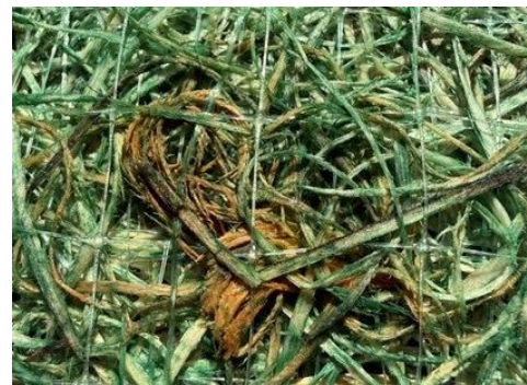
4a & 4b. Mold growth in a competitor's excelsior blanket, including visible dark mold within the fibers. American Excelsior Company minimizes this risk through strict quality controls. Curlex ECBs with QuickGRASS® use an environmentally friendly, malachite-green-free pigment applied to naturally dried Great Lakes aspen fibers. The dry fibers promote even color distribution and help prevent mold growth when properly stored.
