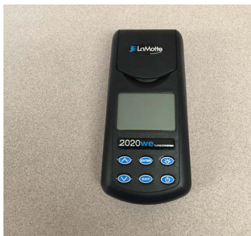
Figure 12. LaMotte 2020we Turbidity Meter used for NTU measurements.
