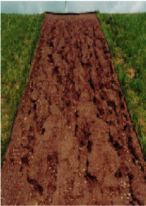
Figure 1. Loam Test Plot Following Storm Series Under Bare Soil Conditions.
