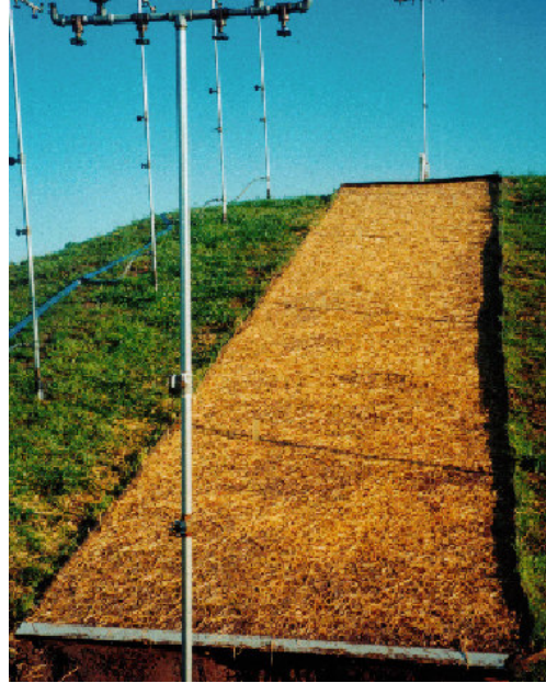
Figure 2. Chetek Sandy Loam Plot Covered With Blown Straw Following Storm Series.
