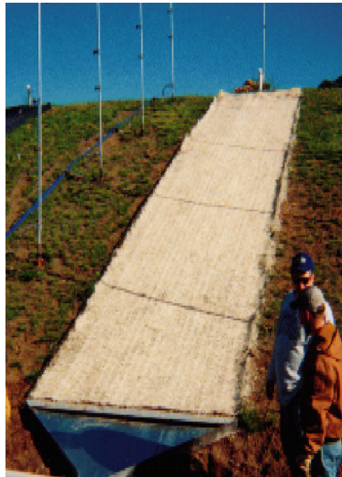
Figure 3. Chetek Sandy Loam Plot Covered With Excelsior Blanket Prior to Testing.
