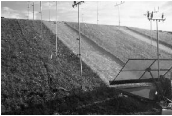
Figure 2. Erosion test plot during the 20.3 cm/hr (6 in/hr) portion of the test series.
