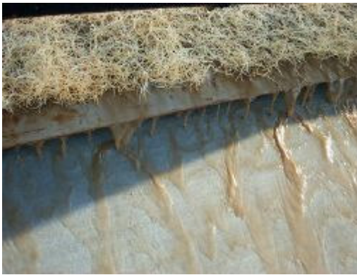
Figure 13. Runoff during the 6 in/hr (152 mm/hr) segment of a double net wood RECP test.
