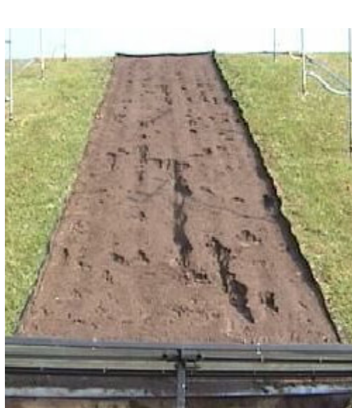
Figure 9. Plot after straw/coconut blanket was removed following the completion of the test series.
