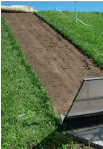
Figure 8. Plot after wood fiber blanket was removed following the completion of the test series.
