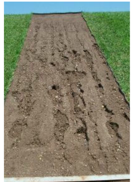
Figure 10. Bare soil control plot following the completion of the test series.
