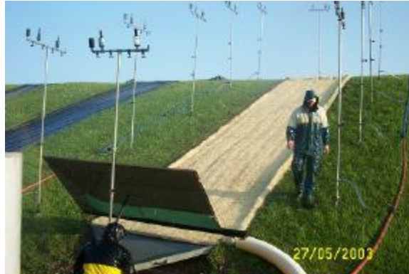
Figure 4. Rainfall simulator in action during the 4 in/hr (102 mm/hr) target intensity segment of a test series.
