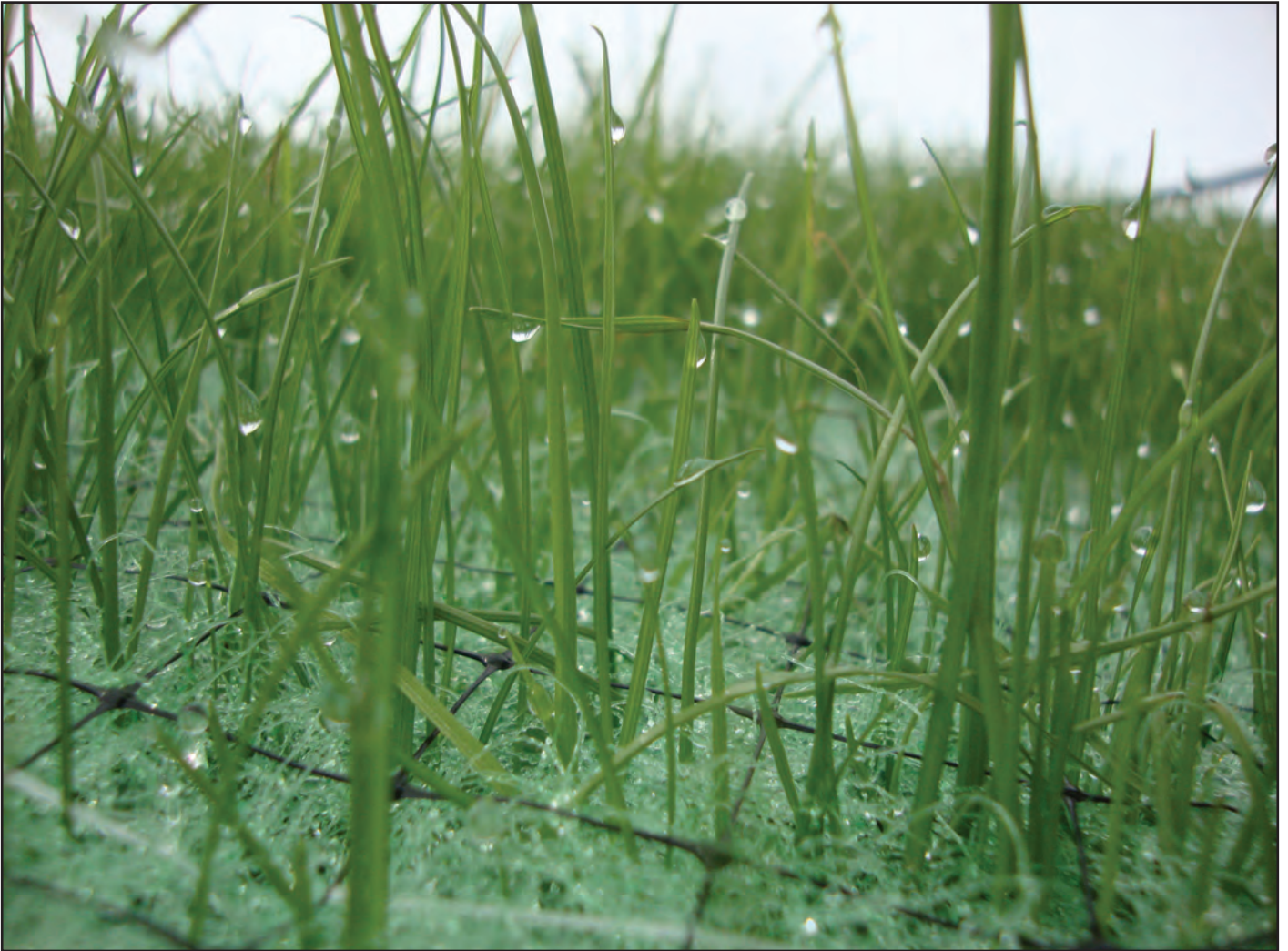
Turf Reinforcement Mats (TRMs) with fibers from 100% recycled post-consumer goods were invented in the early 2000s. Photo courtesy of American Excelsior Company.
