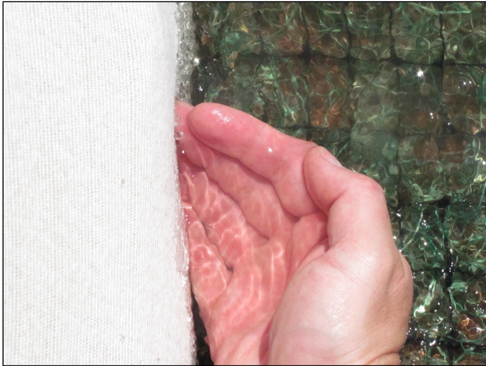
Figure 11. Typical water quality exiting Curlex Bloc filtering station during simulation.
