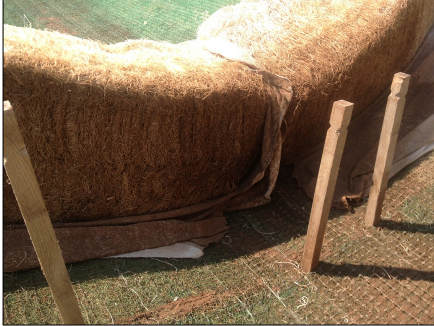
Figure 16. Containment material removed from back bottom Curlex Bloc after simulation.
