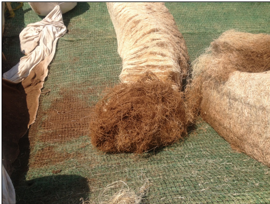
Figure 15. Cross section view of the front bottom Curlex Bloc after containment material was removed following simulation.
