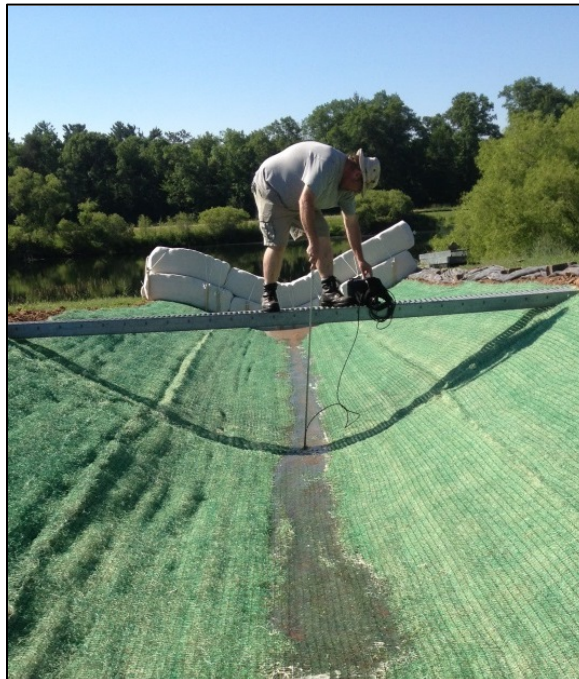
Figure 9. Checking flow velocity shortly after simulation began.
