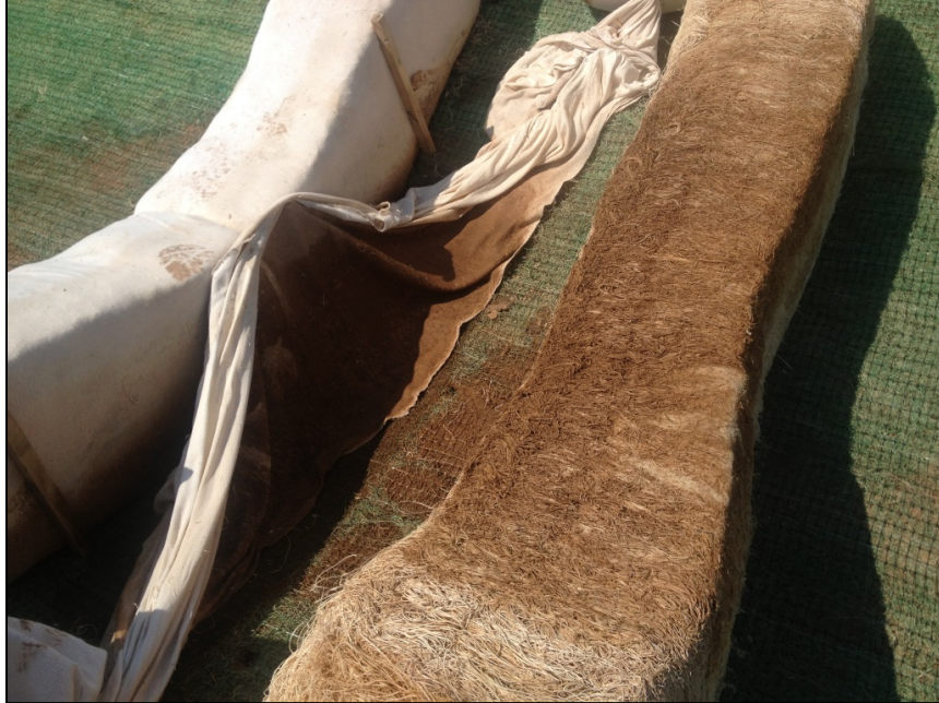
Figure 14. View of the underside of the front bottom Curlex Bloc after containment material was removed following simulation.
