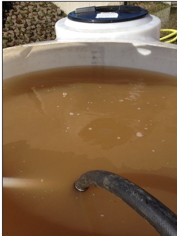
Figure 8. Mixing of sediment-laden slurry in tank before being pumped into channel.
