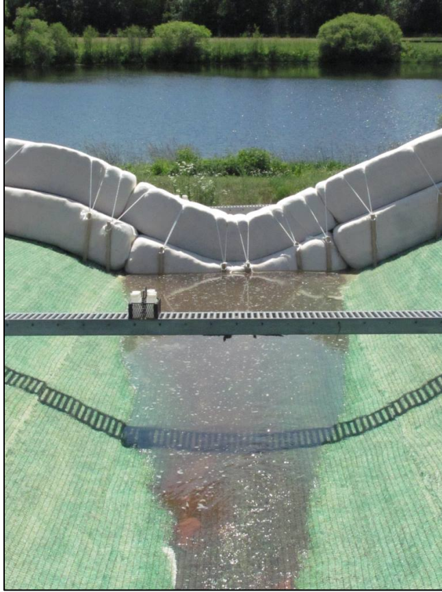
Figure 10. Flow conditions in front of Curlex Bloc filter station near end of four hour simulation.
