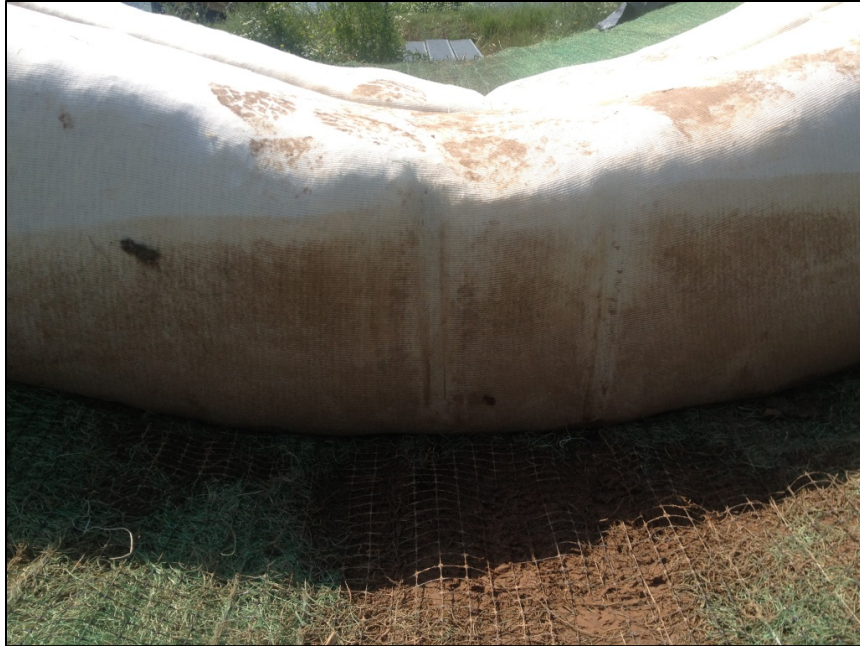
Figure 12. Appearance of front bottom Curlex Bloc after simulation.
