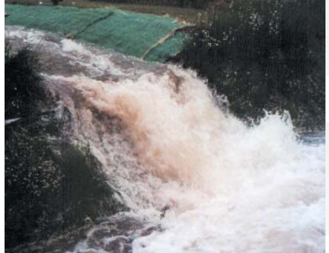
Figure 4. White water exiting test channel after flowing over green QuickGRASS ® .
