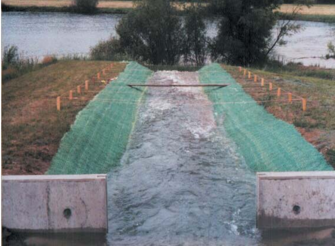
Figure 3. Hydraulic testing of QuickGRASS ® .
