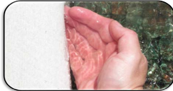
Figure 1. Clear water exiting Curlex Bloc after being filtered by it.
