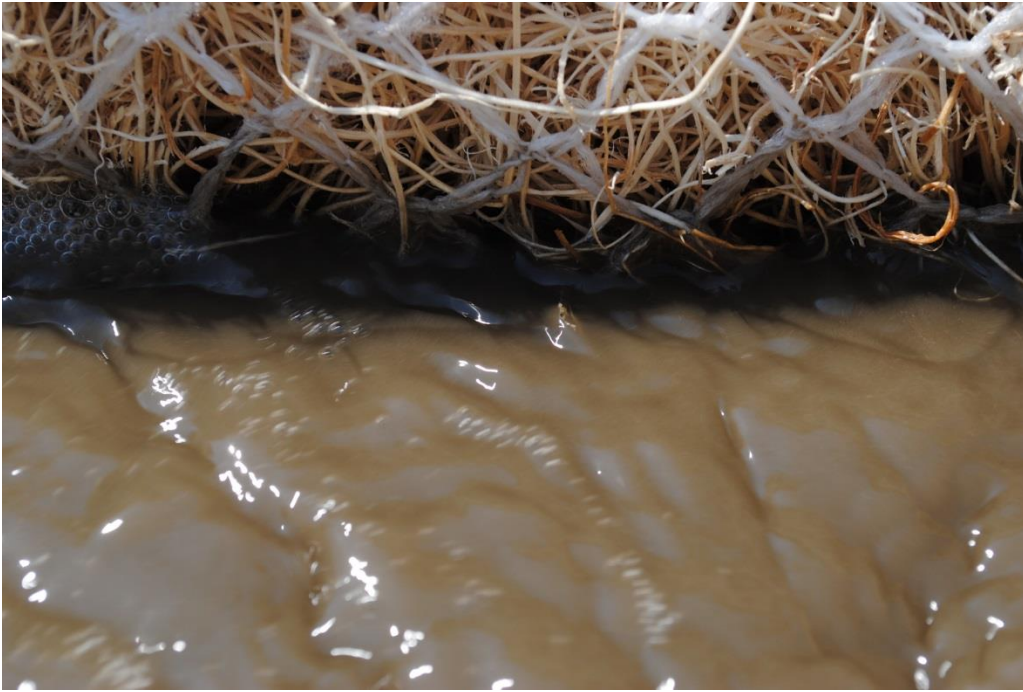
Figure 9. Close up of filtered fly ash slurry exiting a Curlex Sediment Log early in a test.
