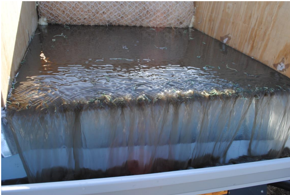
Figure 8. Return channel to supply tank of channel simulator.
