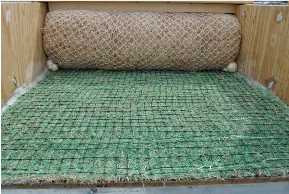
Figure 5. Curlex Sediment Log installed in channel simulator.
