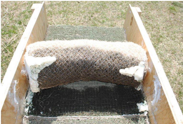
Figure 15. Fly ash on Curlex Sediment Log and between Curlex Enforcer (shown after Curlex Sediment Log was removed from channel bottom following a test).
