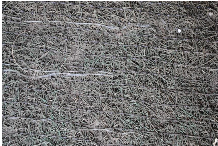
Figure 17. Fly ash within Curlex Enforcer following a filtration test.
