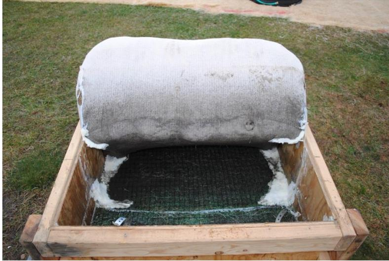
**Figure 15.** Fly ash on Curlex Bloc and between Curlex Enforcer (shown after Curlex Bloc was removed from channel bottom following a test).
