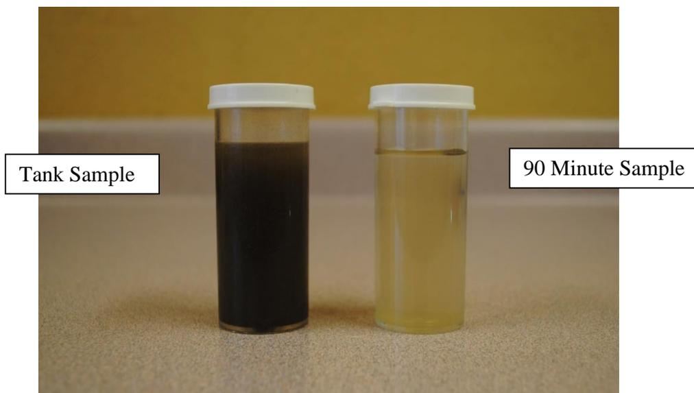
**Figure 18.** Typical turbidity samples showing reduction over time from filtering by Curlex Blocs and Curlex Enforcer.
