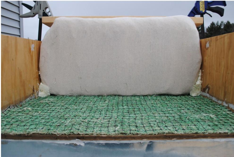
**Figure 5.** Curlex Bloc installed in channel simulator.
