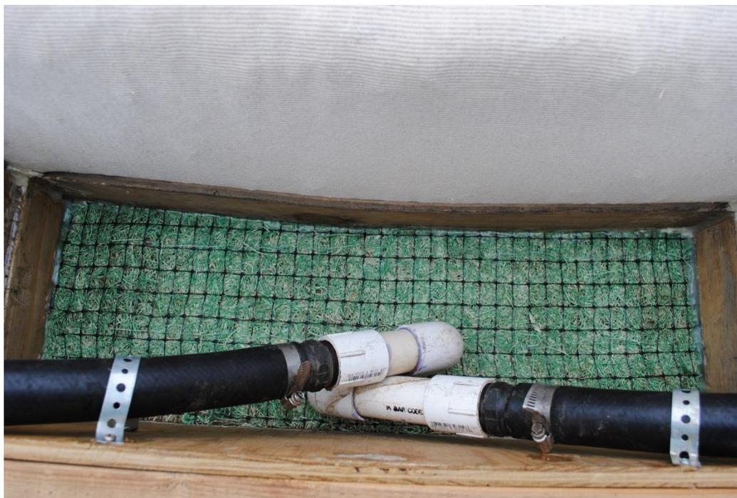
**Figure 6.** Inlet reservoir of channel simulator.
