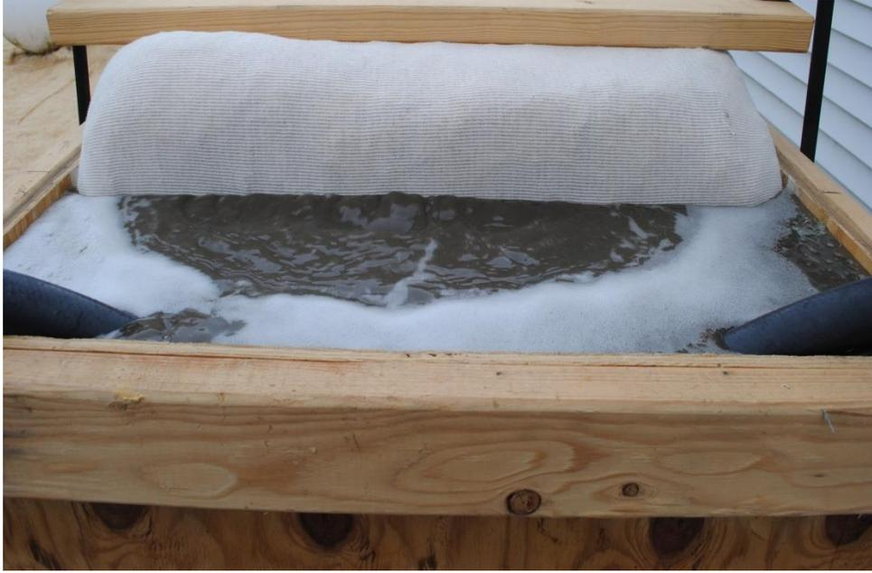
**Figure 7.** Fly ash slurry in the inlet reservoir.
