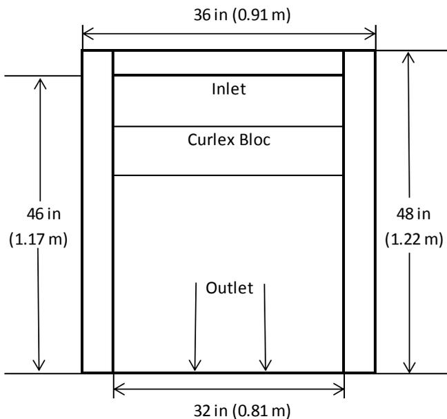
**Figure 2.** Top view of channel simulators.
