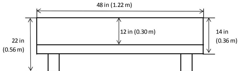
**Figure 3.** Side view of channel simulators.
