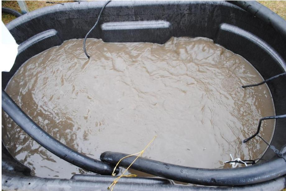
**Figure 1.** Fly ash and water slurry being mixed.
