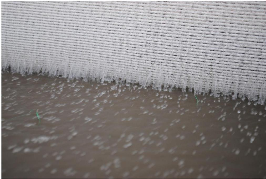
**Figure 9.** Close up of filtered fly ash slurry exiting a Curlex Bloc early in a test.
