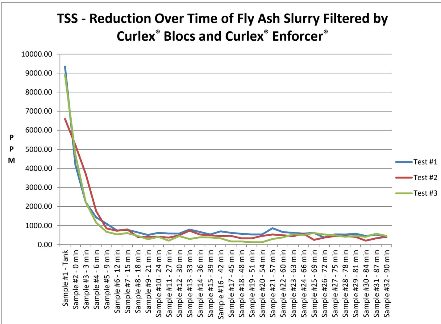
Figure 13 - TSS reduction over time of fly ash slurry filtered by Curlex Blocs and Curlex Enforcer.
