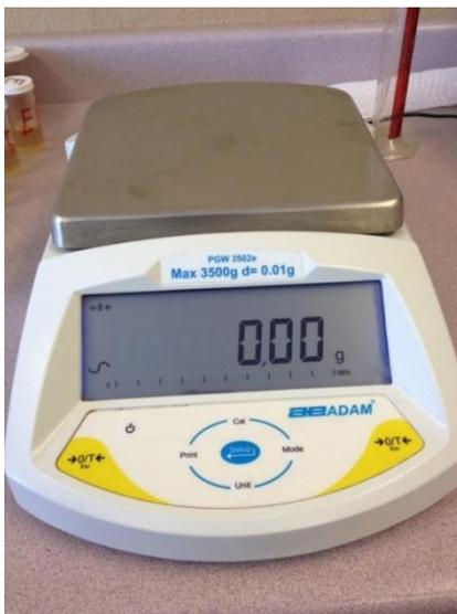
**Figure 11.** Adam Equipment Model PGW 3502e scale used for fly ash mass and TSS analyses.
