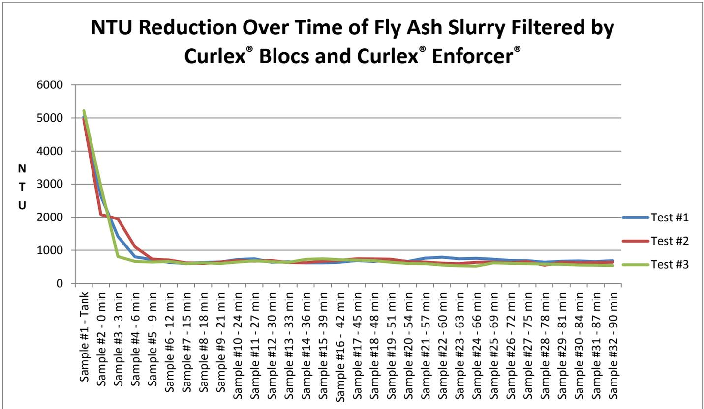
Figure 14. NTU reduction over time of fly ash slurry filtered by Curlex Blocs and Curlex Enforcer.
