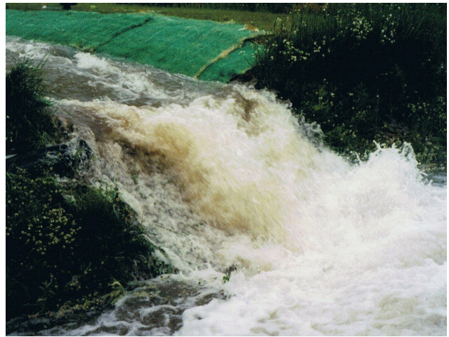
Figure 6. White water exiting test channel flowing over green QuickGRASS.
