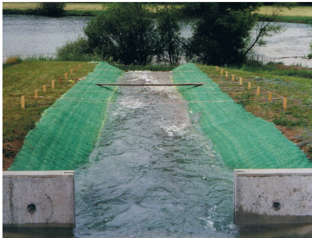
Figure 5. Hydraulic flume testing of QuickGRASS.
