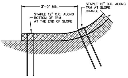
**BOTTOM OF SLOPE TERMINATION IF INSTALLED 3' BEYOND THE TOE OF SLOPE**
