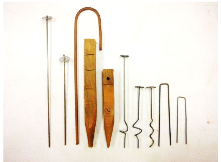
Figure 13: Anchors used in pullout testing.
