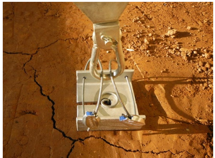
Figure 15: Pullout test of twist style pin in loam soil.
