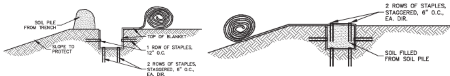
Figure 1: Example Rolled Erosion Control Product (RECP) trench method.
