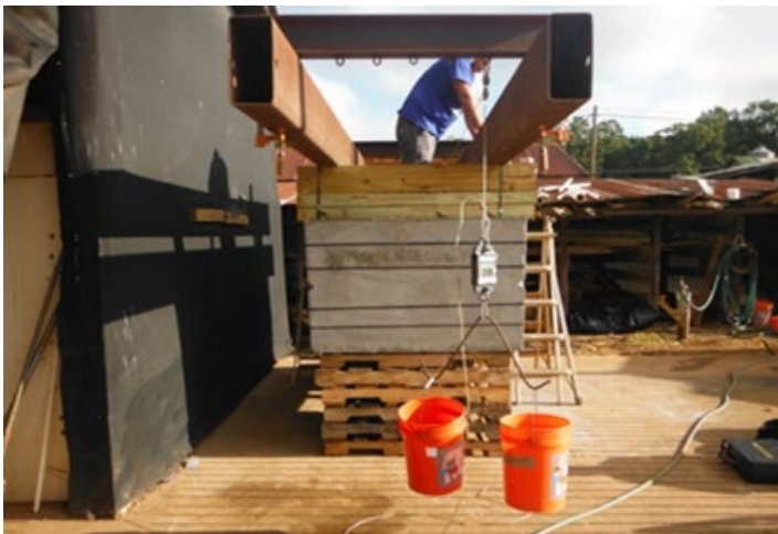
Figure 5: Water vessel hanging on load cell. Photo provided by TRI Environmental, Inc.
