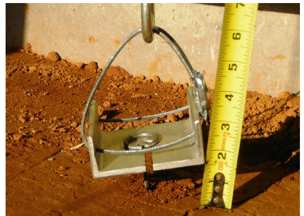
Figure 10: Pullout measured. Photo provided by TRI Environmental, Inc.
