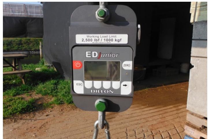
Figure 6: Load cell attached to water vessel and anchor. Photo provided by TRI Environmental, Inc.
