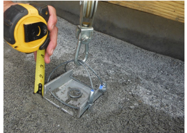
Figure 7: Anchor installed prior to test. Photo provided by TRI Environmental, Inc.
