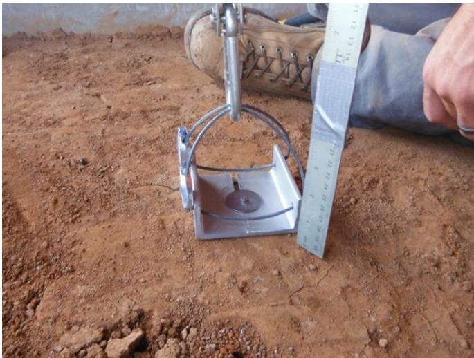
Figure 12: Pullout test of pin with washer in loam soil.
