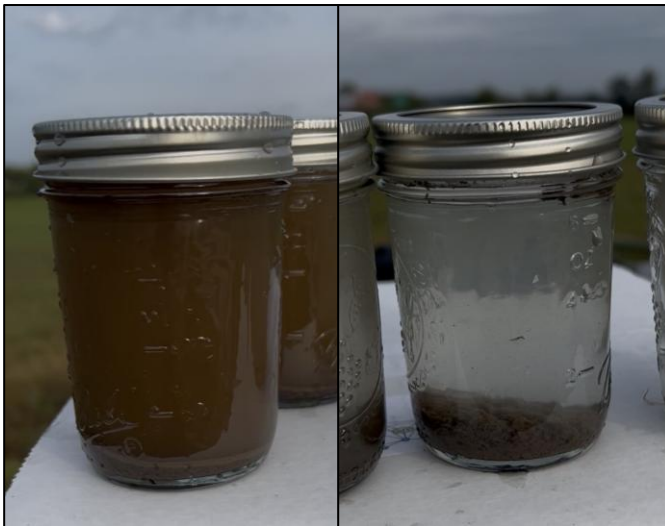
Figure 8: Turbid water samples taken from each end of the channel. Left photo: >300 NTUs. Right photo: ~10 NTUs.
