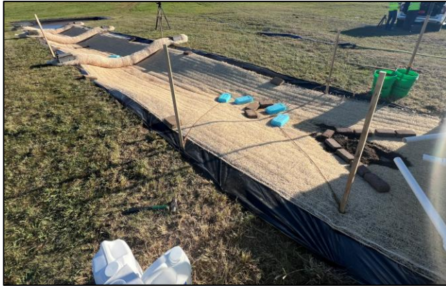
Figure 4: Curlex III FibreNet ECB channel with Curlex Sediment Logs in combination with Floc Logs and Silt Stop powder.
