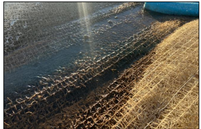
Figure 7: Sediment particles settled onto and captured within the Curlex fiber matrix.
