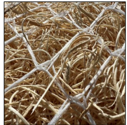
Figure 3: Close-up of Curlex fiber matrix within Curlex Sediment Log.
