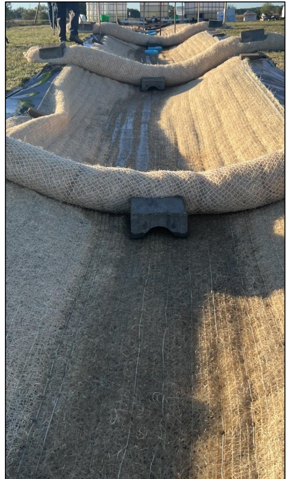
Figure 9: Curlex III FibreNet ECB and APS flocculant products working together to lower NTU values by 97%.
