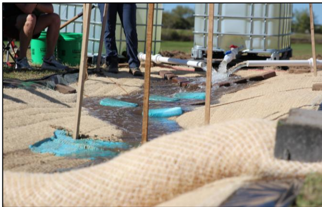
Figure 6: Floc Logs and Floc Log Mat installed with turbid flow over the Curlex III FibreNet ECB and through the Curlex Sediment Log matrix.
