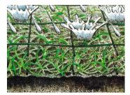
Shock Absorption The mat of Curlex fibers and netting arrests the destructive energy of raindrops, holds soil and seed in place, and helps establish vegetation.
