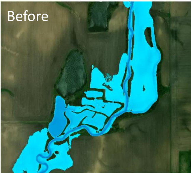
Figure 10. Before improvements, a large portion of the floodplain on the east side of the stream was not connected to the stream. This resulted from a large spoil pile that was left remaining from the gravel mining operation during the 1950s. A large portion of the west flood plain was only connected through water backing up through the remnant gravel pits. Water flowed rapidly across the east side of the flood plain, exiting quickly through a culvert with a flap gate.
