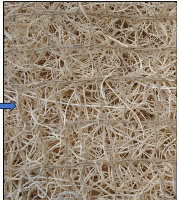
Figure 3: Close-up image of Curlex II FibreNet.
