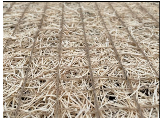
Figure 3: Close-up of Curlex II FibreNet.
