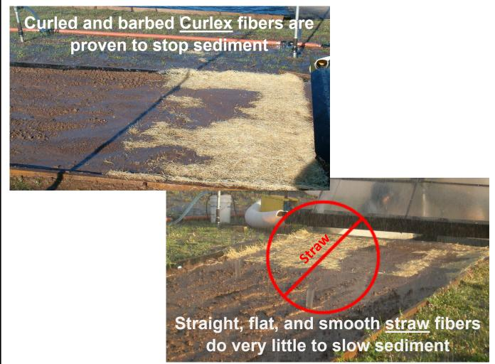
Curlex fibers have a higher Manning's N than straw fibers. This "roughness" provides superior sediment control. Curlex fibers expand when they get wet and dig into the soil. This creates a velcro-like connection for superior erosion control. All Curlex erosion and sediment control products are made from sustainably harvested Great Lakes Aspen and are naturally seed free.
