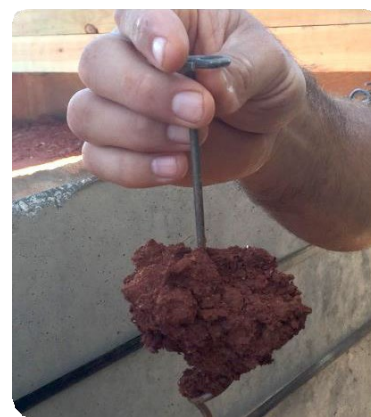
Twist anchor bonds to soil.
