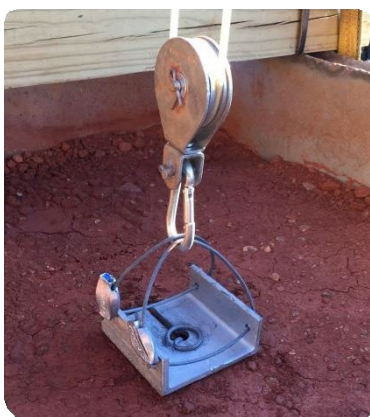
Twist anchor pullout test.
