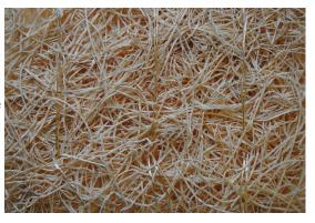
Curlex NetFree ECB is intended for use in low-flow channels. Large scale testing that followed procedures outlined in ASTM D-6460, "Standard Test Method for Determination of Erosion Control Blanket (ECB) Performance in Protecting Earthen Channels from Stormwater-Induced Erosion", showed the ability of Curlex NetFree to protect channels from stormwater-induced erosion. Curlex NetFree will withstand tractive forces  $\leq 1$  lb/ft<sup>2</sup>.
