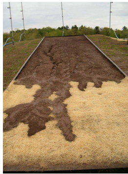
Figure 8. Soil on 2.4 m excelsior buffer strip following test series.
