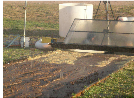
Figure 9. Runoff flowing over 2.4 m straw buffer strip and directly off toe of slope during 15.2 cm/hr segment.
