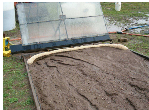
Figure 6. Nearly half the 10.2 cm/hr deposition washed off the plot by the conclusion of the 15.2 cm/hr segment.
