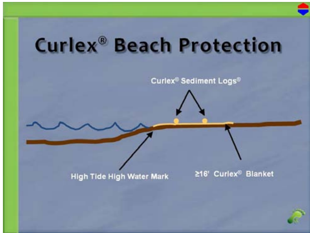
Figure 1. Proposed Curlex beach protection for oil spill response.
