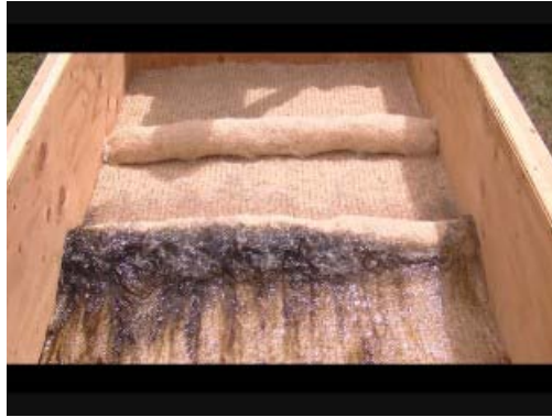
Figure 7. Contaminated water at first Curlex Log.
