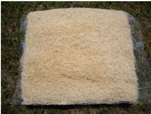
Figure 14. Pad with Curlex fibers between two layers of netting.
