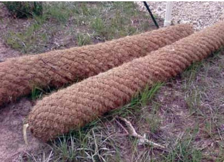
Figure 1. Coir logs are frequently used in shoreline and streambank stabilization.
