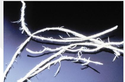
The blankets combine a mat of curled and seasoned Great Lakes Aspen wood excelsior with a tough, photodegradable plastic mesh, which remains in place even on rough terrain. Curlex fibers expand when they become wet. As moisture is released, the fibers contract. This natural motion creates a digging effect that results in superior soil adhesion.
