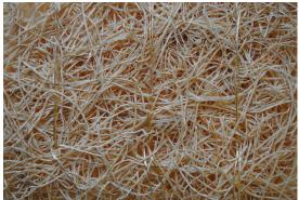
Curlex NetFree ECB is intended for use in low-flow channels. Large scale testing that followed procedures outlined in ASTM D-6460, "Standard Test Method for Determination of Erosion Control Blanket (ECB) Performance in Protecting Earthen Channels from Stormwater-Induced Erosion", showed the ability of Curlex NetFree to protect channels from stormwater-induced erosion. Curlex NetFree will withstand tractive forces  $\leq 1 \text{ lb/ft}^2$ .
