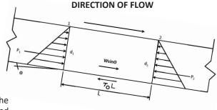
If non-uniform flow conditions are present (i.e. accelerating or decelerating flow) or if channel cross section changes are encountered, a more sophisticated analysis will be required. Special attention needs to be given to hydraulic structures, such as bridges and culverts. For most cases, the above equation is applicable.
