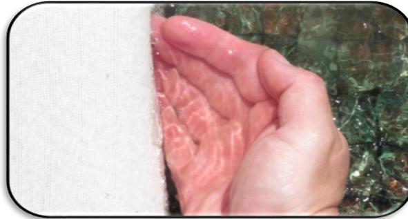
Figure 1. Clear water exiting Curlex Bloc after being filtered by it.
